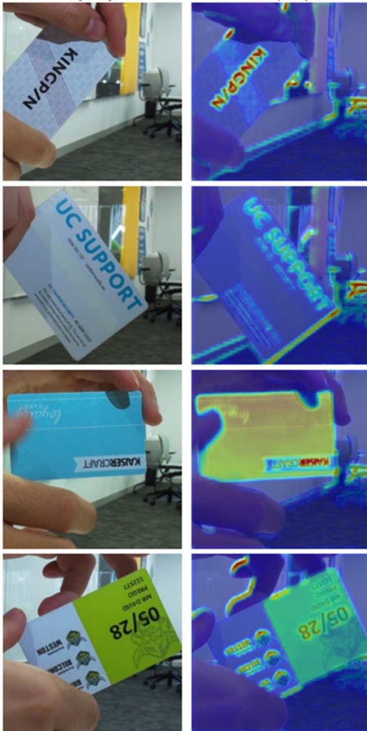
Figure 6: Samples of the Grad-CAM heatmaps indicating the regions of the image that have the most impact on the model's classification predictions
